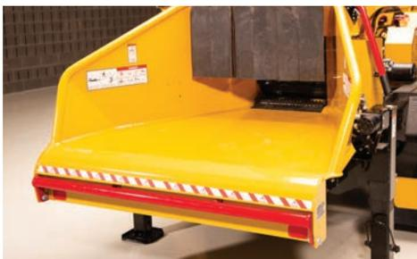
**ROBUST FEED TABLE.** Mechanized feeding made effective with a wide feed roller opening and durable, fixed infeed table design.
