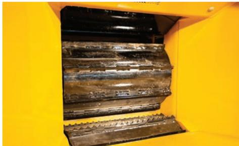
**INTELLIGENT FEED SYSTEM.** Providing over 6,500 lb (2,948 kg) of pull-in power, the AX17 uses SmartCrush and SmartFeed control system that reduces the need for operator interaction when feeding difficult material.
