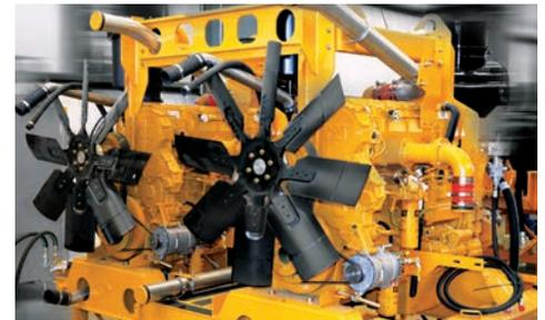
**ONE CAT IS NOT ENOUGH.** The T1655III features two CAT C18 ACERT engines providing 1200 hp (895 kW) to muscle through the toughest conditions.
