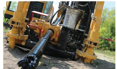
**LESS RESTRICTIONS.** A hollow inner rod design results in more air and drilling fluid flow to the drill head on pilot bores and the hole opener during pullback, providing contractors the ability to select from a more diverse range of tooling options, including air hammers and larger hole openers.
