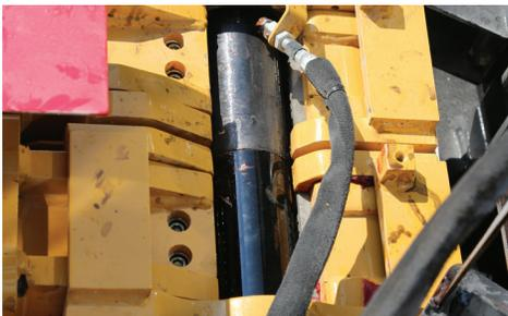
**REDUCED STEPS.** The time and steps required to add or remove a rod on the D40x55DR S3 is significantly less than previous Vermeer models due to an enhanced dual drill rod design that quickly and easily makes up the inner and outer rod connections.
