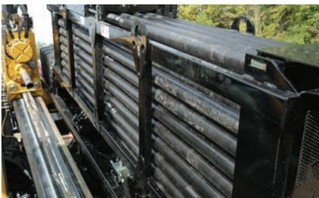
**MORE FEET ONBOARD.** Install more feet and save time with an impressive 500 ft (152.4 m) of drill rod on-board.
