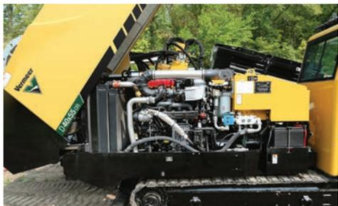
**IMPRESSIVE POWER.** Powered by a 140 hp (104 kW) John Deere diesel engine, this drill serves up 40,000 lb (177.9 kN) of thrust/pullback and 5,500 ft-lb (7,457 Nm) of rotational torque.
