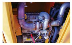
**EASE OF MAINTENANCE.** The TR5300 features a maintenance access platform for the Deutz TD 2.9L Tier 4 Final (Stage IV), 74 hp (55 kW) engine. With several access doors around the engine compartment, maintenance work on vital machine systems can be completed with minimal effort.
