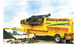
**GRIZZLY SCREEN OPTION.** The optional grizzly attachment can be mounted over the hopper to prescreen large materials and create more consistent overs material.
