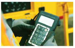
**CONVENIENT CONTROL.** Operators can control the machine through either the machine display mounted on the control panel, or through a transceiver remote. From either control, the operator can choose from four programmable presets or adjust on the fly based on incoming material.
