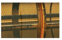
**PRODUCT VARIETY.** Change product sizing more efficiently with the quick-change screen design. Five large bolts adjust a tensioning hook to allow operators to quickly change screen sizes.
