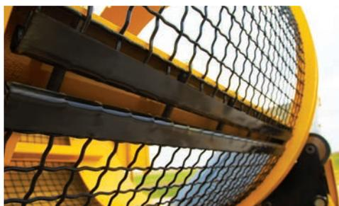
**PRODUCT VARIETY.** Change product size more efficiently with the quick-change screen design. Five large bolts adjust a tensioning hook to allow operators to quickly change screen sizes.
