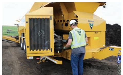
**BUILT FOR EASE OF MAINTENANCE.** The TR6400 has various access points to critical areas which allows the operator to efficiently maintain the machine.
