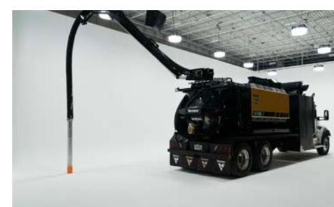
**SIDE STOW BOOM.** Minimizes setup time by keeping the dig tube connected at all times - even during transport - operators can move work done in a day.
