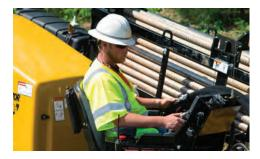
**SIGNIFICANT SOUND REDUCTION.** With a 104 dB(A) guaranteed sound power level and an operator ear rating of 82.9 dB(A), as well as an in-cab operator ear rating of 75.7 dB(A), the D24x40 S3 contributes to a quieter working environment, creating less neighborhood disturbance and enabling easier communication among the crew.
