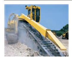
**Track Trenching:** Because the Terrain Leveler SEM drum is an attachment, the base tractor can be switched to a trencher cutting boom. Track trenching will allow the unit to work in mainline sewer and water applications — maximizing the use of the tractor unit.
