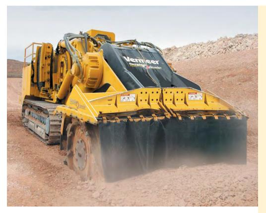
One Vermeer T1255 Terrain Leveler SEM can perform overburden removal and THEN surface mine in very specific layers. Blasting and rippers are unnecessary, and the material is ready for transport without any additional sizing steps.
