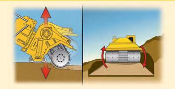
A patented, industry-exclusive tilting cutter drum with two-direction leveling on the T1255 aids production by keeping the drum level — allowing the unit to take on jobs that were not possible before — regardless of ground conditions. It also offers the ability to utilize laser guidance to control grade.
