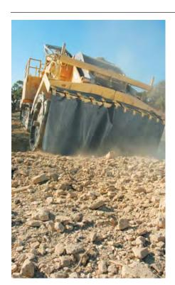
**Road Construction / Reconstruction:** Terrain Leveler surface excavation machines offer a great way to excavate rocky areas in preparation of new roads. They also provide an excellent method for roughing out house pads in new construction.
