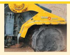
**Proprietary top-down cutting technology** allows the cutter teeth to achieve greater rock penetration. When the machine travels forward, the teeth on top of the drum are positioned over the top of the rock surface. As contact is made, the teeth instantly cut the rock.
