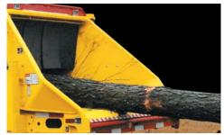
SMART CRUSH. Once the upper feed roller freely raises for four seconds, it will automatically increase down pressure on the material being fed. This allows the upper feed roller to easily climb onto large forked material before the increased down pressure is applied for maximum pulling force.
