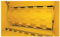
LOWER FEED ROLLER. The lower feed roller is offset from the upper feed roller by 10.8" (27.4 cm). Material is easily pulled to the upper feed roller, so there is less need to manually raise the upper feed roller for larger diameter material.
