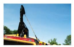
**OPTIONAL WINCH.** Eliminates the need to drag large material to the chipper. The 150' (45.7 m) winch line can handle material up to 4000 lb (1814.9 kg), making it easy to lift logs directly onto the feed table. In addition the winch can also be hydraulically raised out of the way to allow operators to feed the unit using a loader. Vermeer
