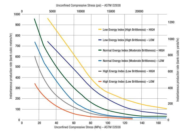
Production rates shown on this chart have been determined through field trials. Before the trials occurred, rock samples were submitted to the Vermeer Rock Lab for analysis. These results were then correlated with the corresponding production rates.
