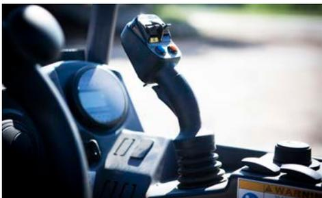
**MULTIFUNCTION JOYSTICK.** The multifunction joystick utilizes electric-over-hydraulic toggles for ease of access to machine functions like the telescopic boom, auxiliary hydraulic controls and the Dynamic Blocking System (DBS). The operator does not have to remove their hand from the loader arm controls in order to function any of these features.
