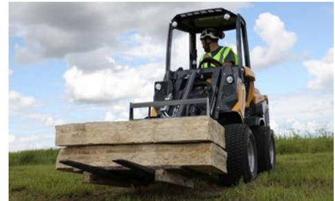
**LIFT-TO-WEIGHT RATIO.** The ATX850 has a rated operating capacity (straight) of 1,590 lb (721 kg)\* while having a standard weight of 4,254 lb (1,930kg) with rear weights and without attachments. This lift-capacity-to-weight ratio allows contractors to utilize a lighter machine while still being able to carry heavy materials on the jobsite.
