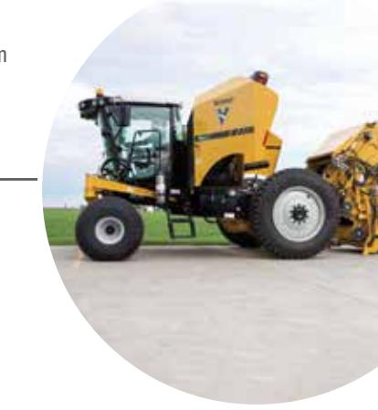
**5** The bale chamber can be removed for quick maintenance. After the chamber is detached from the base unit, operators have convenient access to the bale chamber for routine maintenance.
