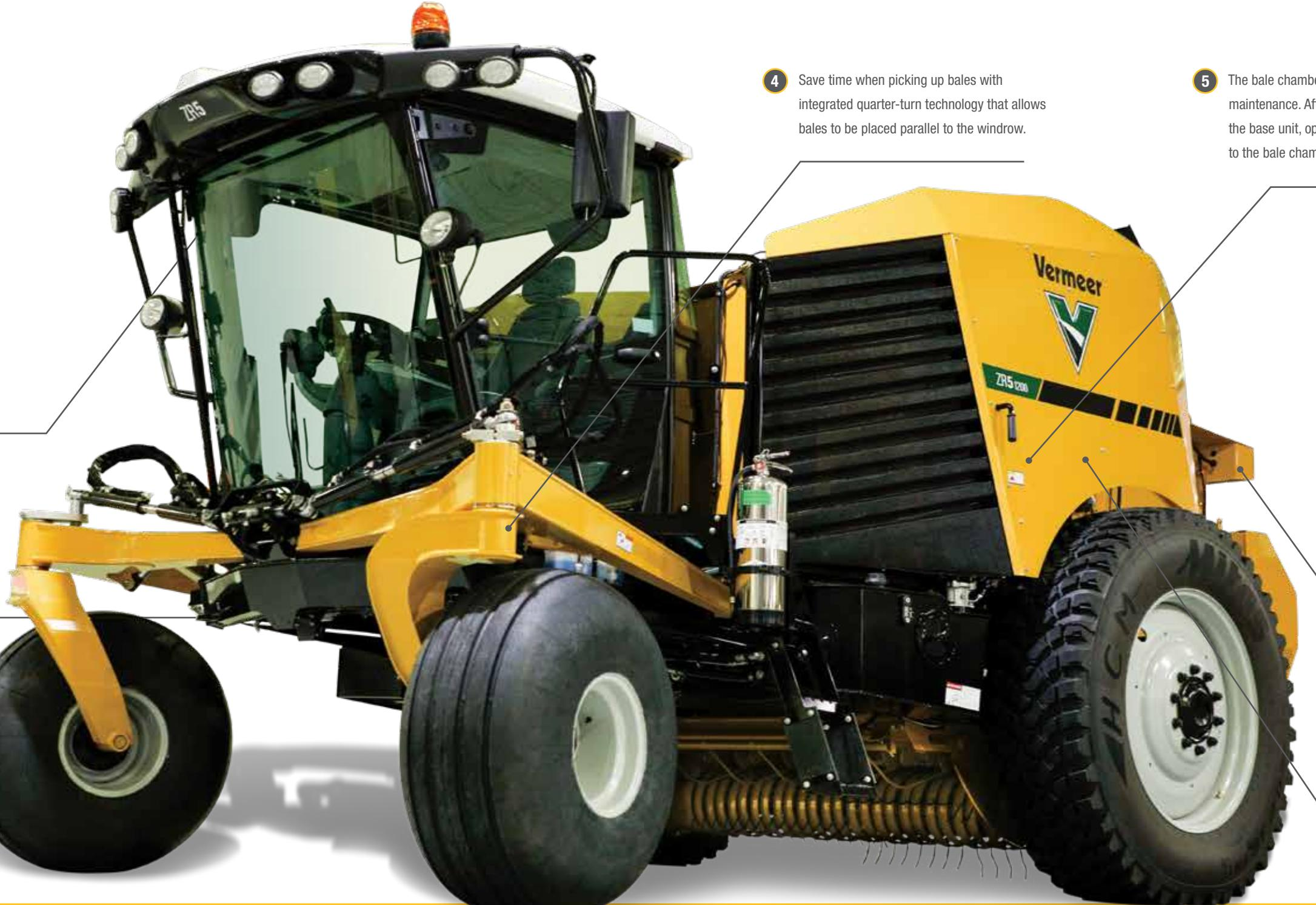
**4** Save time when picking up bales with integrated quarter-turn technology that allows bales to be placed parallel to the windrow.
