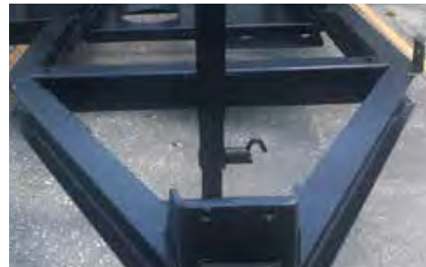
I BEAM TRAILER. Units are built from start to finish at our factory, including the trailer which consists of a sturdy I beam construction.
