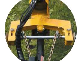
6 A patented 2-point Quick Hitch hookup is designed to allow one person to hook up the mower. It also provides high ground clearance to help avoid obstructions while in the field.
