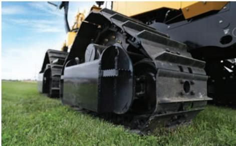
**STEEL QUAD TRACK SYSTEM.** Four independent steel tracks can offer enhanced floatation and traction with four-wheel and crab steering options.
