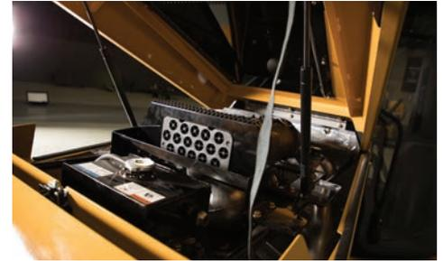
**POWER FOR THE JOB.** The XTS1250i2 is powered by a 127 hp (95 kW) Deutz TCD3.6L diesel engine which offers efficient power for working in difficult ground conditions.
