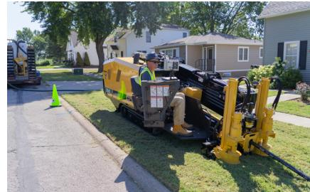
**PRICED RIGHT AND SIZED RIGHT.** The D20x22 S3, smallest drill in its class, is well-suited to install cable, fiber and product pipe efficiently and productively in a small footprint, without outpricing what you need for the market.
