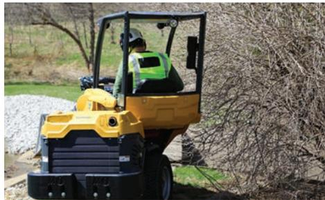
**COMPACT SIZE.** With narrow tires, the ATX530 is 40.9-in (103.9 cm) wide, while the wider tires make the machine 47.2 in (119.9 cm) wide. Both configurations allow the ATX530 to fit through a standard four-foot gate for backyard access on landscape jobs. The overall length of the ATX530 is 98.4 in (249.9 cm).
