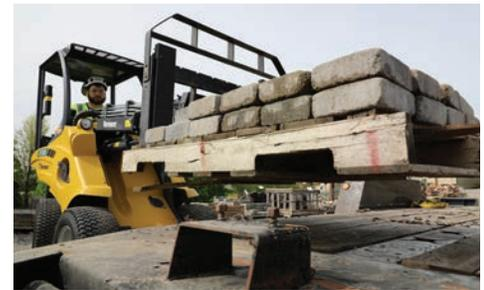
**LIFT-TO-WEIGHT RATIO.** The ATX530 has a rated operating capacity (straight) of 1,492 lb (677 kg)\* while having a standard weight of 2,756 lb (1,250 kg) with rear weights and without attachments. This lift-capacity-to-weight ratio allows contractors to utilize a lighter machine while still being able to carry heavy materials on the jobsite.
