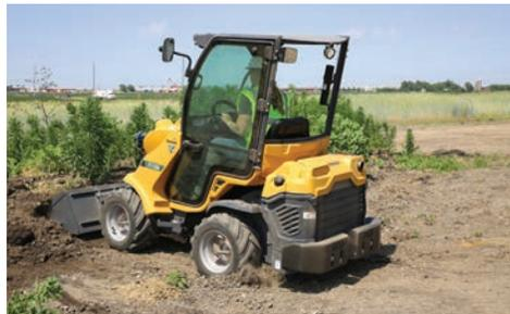
**FOURWHEEL DRIVE HYDROSTATIC DIRECT DRIVE MOTORS.** As each wheel has a hydrostatic direct drive motor, hydraulic oil can flow freely to each wheel as needed during transport which helps reduce ground disturbance on turf when making turns. The fourwheel drive hydrostatic direct drive motors also allow for the use of the DBS and torque divider to increase tractive effort in difficult conditions.
