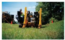
WHEN THERE'S A JOB TO BE DONE. With 28,000 lb (124.6 kN) of thrust/pullback and 4,200 ft-lb (5694.4 Nm) of rotational torque, the D24x40 S3 offers an increase over its predecessor, helping to maximize machine and jobsite productivity.
