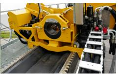
**EXTENDED DRILL PIPE RANGE.** The vise travels the full length of the rack, delivering 220 kNm of breakout torque and 110 kNm of makeup torque. This allows the use of drill pipes with an outer diameter of up to 7.625 in (194 mm). Its large passthrough opening supports tooling and steel casing with outer diameters up to 406 mm (16 in), providing enhanced versatility for demanding drilling operations.
