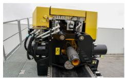
**UNMATCHED DRILLING POWER.** With an impressive peak torque of 110 kNm, the D120E rivals the performance of larger maxi rigs. Its advanced direct electric drive delivers swift responsiveness, pinpoint control and scalable power maximizing efficiency across every phase of operation.
