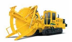
**HYDROSTATIC ROCKWHEEL ATTACHMENT.** Powered by dual hydrostatic motors, the rockwheel attachment has the ability to cut a trench up to 54" (137.2 cm) in depth and width options of 6", 8", 10", 12" and 14" (15 cm, 20 cm, 31 cm and 36 cm).
