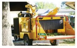
**OPTIONAL WINCH.** The winch allows operators to move large logs with less effort. The 150' (914.4 cm) winch line has 2000 lb (907.2 kg) of pulling force.
