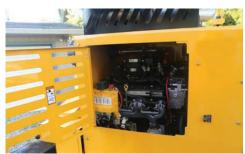
165 HP INDUSTRIAL GAS ENGINE. The BC1800xL is designed with a 165 HP (123 kw) PSI 5.7 L gas engine, powerful enough to tackle jobsite challenges when chipping large diameter wood.
