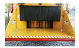
SMOOTH FEEDING. Vertical feed rollers with helical cleats help hold material firmly to the feed table, which helps reduce vibration, shock and structural loading to the rear of the machine.
