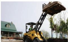
**TELESCOPIC BOOM.** The telescopic boom on the ATX530 extends 21.6 in (54.9 cm) for loading materials to a dump height of 108.3 in (275.1 cm) in hinge pin height. The telescopic boom can also aid in dumping material over the backside of a retaining wall or grabbing material over an obstruction.
