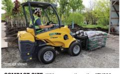
COMPACT SIZE. With narrow tires, the ATX530 is 40.9-in (103.9-cm) wide, while the wider tires make the machine 47.2-in (119.9 cm) wide. Both configurations allow the ATX530 to fit through a standard four-foot gate for backyard access on landscape jobs. The overall length of the ATX530 is 98.4 in (249.9 cm).
