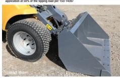
**MULTI-TOOL ATTACHMENT PLATE.** The ATX530 can be fitted with various authorized attachments to meet the jobsite need, may that be for snow removal, landscaping and tree care work, or various other applications.
