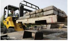
LIFT-TO-WEIGHT RATIO. The ATX530 has a rated operating capacity (straight) of 933 lb (423.2 kg)\* while having a standard weight of 2711 lb (1229.7 kg) with rear weights and without attachments. This lift-capacity-to-weight ratio allows contractors to utilize a lighter machine while still being able to carry heavy materials on the jobsite.
