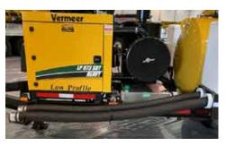
**SIDE HOSE AND TOOLING (SHT) STORAGE (OPTION).** The new SHT package allows for 60 ft (18 m) of suction hose storage on a trailer-mounted unit. This doubles the traditional 30-ft (9-m) hose storage on all other brands.
