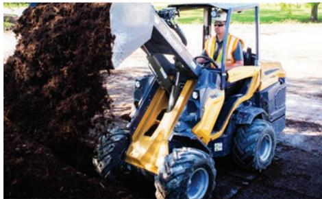
**COMPACT SIZE.** With narrow tires, the ATX850 is 42.1-in (106.9-cm) wide, while the wider tires make the machine 50.4-in (128-cm) wide. Both configurations allow the ATX850 to fit through a standard four-foot gate for backyard access on landscape jobs. The overall length of the ATX850 is 120.3 in (305.6 cm).
