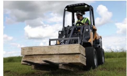
**LIFT-TO-WEIGHT RATIO.** The ATX850 has a rated operating capacity (straight) of 2,542 lb (1,153 kg)\* while having a standard weight of 4,254 lb (1,930kg) with rear weights and without attachments. This lift-capacity-to-weight ratio allows contractors to utilize a lighter machine while still being able to carry heavy materials on the jobsite.
