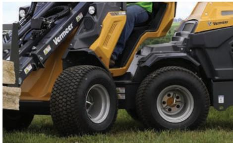
**FOUR WHEEL DRIVE HYDROSTATIC DIRECT DRIVE MOTORS.** As each wheel has a hydrostatic direct drive motor, hydraulic oil can flow freely to each wheel as needed during transport to help reduce ground disturbance on turf when making turns. The four wheel drive hydrostatic direct drive motors also allow for the use of the DBS and torque divider to increase tractive effort in difficult conditions.
