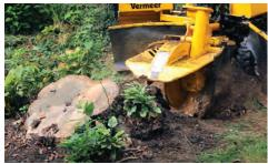
MAXIMUM CUTTING WIDTH. The SC552 reduce the operator's time repositioning the machine with a cutting height of 31" (78.7 cm) above ground and 25" (63.5 cm) below grade. the straight-line cutting dimension allows the operator to cut a 6' (1.8 m) stump without repositioning the machine.
