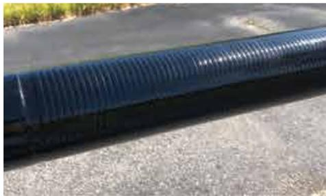
**RIBBED TOOL BODY.** Maximizes production by placing additional friction between the tool body and the surrounding soil. Inside body bore is honed and precision fit to the striker, plus optimized power and wear ring life.
