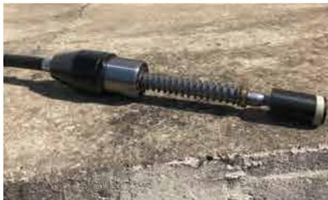
**ALL-STEEL, AIR-ON QUARTER TURN REVERSE.** Allows the operator to efficiently rotate the air hose a quarter turn to reverse the tool. Instant positive audio and visual feedback indicates the tool has shifted into reverse—no need to shut the tool off underground.
