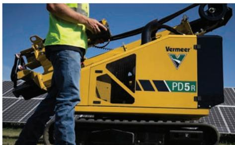
**COMPACT DESIGN.** A small machine with transport dimensions of 85 in (215.9 cm) wide, 8.2 ft (2.5 m) tall and a 15 ft (4.6 m) mast is ideal for jobsites with less space, or for multiple smaller jobs that require continual transportation of the machine. Quickly move around the jobsite and continue efficiency of installations, helping reduce time spent on setup, teardown and transportation.
