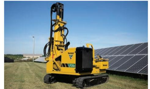
**KEEP IT LIGHT.** The PD5R weighs in at 10,330 lb (4,685.6 kg), which allows for transporting up to two pile drivers on select trailers, and less potential damage to jobsites, all while helping increase efficiency of setup and teardown with a lightweight design.
