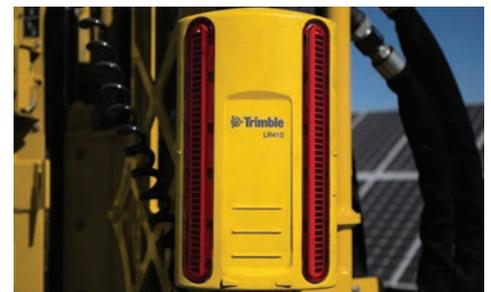
**MAINTAIN ACCURACY.** An optional laser receiver and an optional compatible third-party GPS system can provide visual input to the operator and input to the machine control system to help improve productivity and alignment of the machine to the specified pile location.
