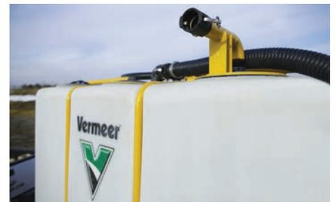
**SERVICEABILITY.** Maintain machine performance with efficient ways to manage necessary components. The occasional replacement of roll jets is made convenient with access through the top of the tank, as well as convenient access to engine and pump service components. Daily tasks such as filling and draining are made convenient with a freshwater fill feature and two valves for system draining.
