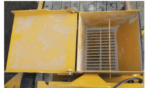
**A CLEAN MIX.** A suction hose and wide-mouth hopper pairs with the tapered bottom rectangular tank to help prevent drilling fluid additives from settling, assist with drainage and reduce buildup.
