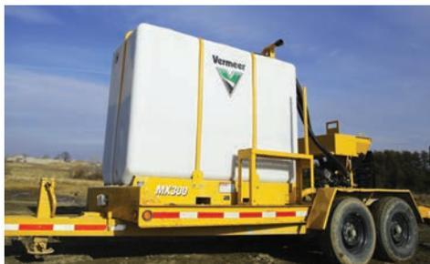
**SLIM FIT.** The MX300 has a tank design that is 105" (266.7 cm) long and 40" (101.6 cm) wide. This slim rectangular profile allows for convenient transport of up to two tanks inside an enclosed truck.
