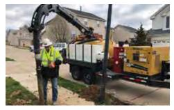
**HYDRAULIC BOOM (OPTION).** The hydraulic boom offers a 6-way function, wireless remote with vacuum valve operation, 330-degree rotation, remote water jet for ease of cleanout, and a 5-in (13-cm) hose with quick connect to 4-in (10-cm) tooling.
