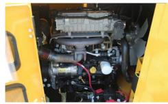
**DEUTZ G2.9 GASOLINE ENGINE.** A 72.4 hp (54kW) Deutz G2.9 gasoline engine designed for demanding industrial applications.
