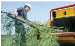
**SMARTFEED.** A patented feedsensing control system which monitors engine rpm and automatically stops and reverses feed rollers when feeding large, hardwood material. With a simple switch, an operator can choose between three rpm droop settings to fit the specific job application.
