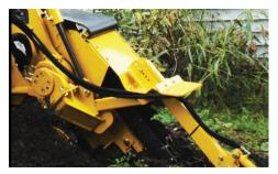
MAKE SENSE OF YOUR TRENCH. When difficult conditions are encountered while trenching, causing a sudden drop in engine speed, the TrenchSense<sup>™</sup> electronic control system automatically pauses the forward motion of the tractor to prevent engine shutdown and recalibration of the machine controls. Once preset engine and trencher speed recovers, forward auto creep resumes. The sequence occurs within seconds and requires no operator adjustment.
