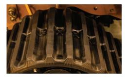
**QUAD TRACK SYSTEM.** The quad track system offers improved flotation, reduced surface damage and increased tractive effort. Four-wheel steer and crab steering are functional with both quad track and rubber tire options.
