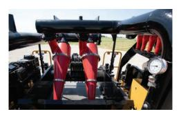
**OPTIMAL RECYCLING PERFORMANCE.** Two 10-in (25.4-cm) desanders and 16 5-in (12.7-cm) desilter hydrocylones remove sand and coarse silts prior to the next stage in the cleaning process, resulting in dry solids.
