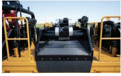
**ENHANCED SHAKER DECK.** Redesigns of the linear motion shaker deck weldment and wedge retention component help reduce weight, increase the available G-force and extend the expected screen life.
