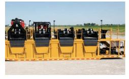
MAXIMUM TANK CAPACITY. A three-tank unit offers a total capacity of 7729 gal (29,257.4 L). A scalped tank, a middle tank and a clean tank combined with a three stage cleaning process help provide a solution that processes over 1100 gpm (4163.9 L/min), with true cleaning capacity suited for horizontal directional drilling (HDD) projects in the 600 gpm (2271.3 L/min) range.
