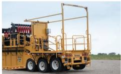
POWER FLEXIBILITY. Contractors can configure the reclaimer with or without the generator set mounted onboard. The option without the generator set onboard includes electrical cables for efficient connections. Contractors have the flexibility in both configurations, and the option to lease or own the generator set.
