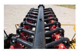
**DESILTER MANIFOLD.** The engineered manifold provides an efficient flow of processed drilling fluid exiting the hydrocyclone, which helps reduce turbulence and excessive vacuum for efficient separation of sands and course silts.
