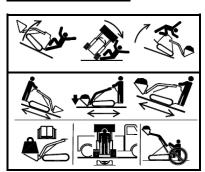
**WARNING:** Traveling on slopes or with load elevated may result in tip over. Serious crushing injury or death can result.
