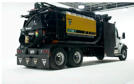
**SIDE STOW BOOM.** Minimizes setup time by keeping the dig tube connected at all times - even during transport - operators can more work done in a day.
