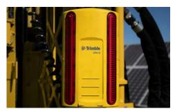
MAINTAIN ACCURACY. The PD5 has an optional laser receiver and an optional compatible third-party GPS system that can provide visual input to the operator, which can help improve productivity and alignment of the machine to the specified pile location.
