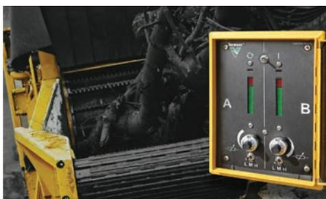
**CONTAMINATION DEFENSE.** The optional Vermeer-exclusive Damage Defense system helps reduce the likelihood of certain metal contaminants from entering the hammermill by reversing the infeed and turning off the feed system when it senses the initial metal contact. These metal contaminants entering the hammermill can damage the machine, so the Damage Defense system helps keep the machine productive by stopping certain metal contaminants from being processed.
