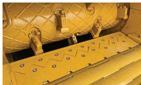
**ANVIL.** The anvil provides the cutting action between the grinder drum or chip drum, and helps break apart the material. The anvil mount structure has been redesigned to handle the high horsepower. This redesign eases the replacement process of the hard-faced wear edge, which results in less time required for maintenance.
