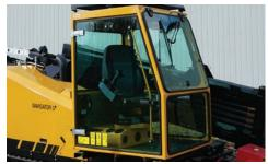
OPTIONAL COMFORTABLE CAB. The excavator-style cab with heating and air conditioning provides operator comfort.
