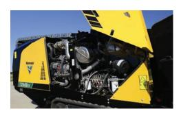
PREMIUM POWER. A 100 hp (75 kW) Deutz TCD3.6L4 engine provides power to help drive the D23x30pr S3 to its peak performance, while a thrust/pullback of 24,000 lb (106.8 kN) combines with rotational torque of 3,000 ft-lb (4067.5 Nm) to help get the drill into tough ground.
