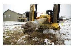
TOUGH TOOLING. With the 2-degree bend positioned in the forward section of the tool, the new greaseable RH10 drill head offers responsive steer on command for precise installations.
