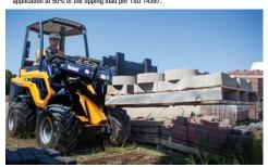
**MULTI-TOOL ATTACHMENT PLATE.** The ATX850 can be fitted with various authorized attachments to meet the jobsite need, may that be for snow removal, landscaping and tree care work or various other applications.
