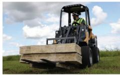
LIFT-TO-WEIGHT RATIO. The ATX850 has a rated operating capacity (straight) of 1,590 lb (721 kg)\* while having a standard weight of 4,254 lb (1,930kg) with rear weights and without attachments. This lift-capacity-to-weight ratio allows contractors to utilize a lighter machine while still being able to carry heavy materials on the jobsite.
