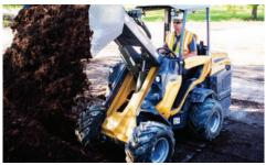
**COMPACT SIZE.** With narrow tires, the ATX850 is 42.1-in (106.9-cm) wide, while the wider tires make the machine 50.4-in (128-cm) wide. Both configurations allow the ATX850 to fit through a standard four-foot gate for backyard access on landscape jobs. The overall length of the ATX850 is 120.3 in (305.6 cm).
