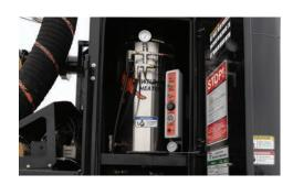
BOILER. 420K BTU diesel fired boiler with coils rated at 5,000 psi (34,473 kPa).
