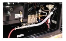
WATER SYSTEM. The water system is rated for 11.5 gpm @ 3,000 psi (43.5 L/min @ 20,684 kPa).
