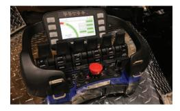
IFM ELECTRONICS. Industry leading IFM industrial controller that monitors the systems temperature, pressure and vacuum sensors. It also allows the operator to see the engine instruments, the chassis instruments, as well as the vac instruments on the belly pack.
