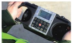
**REMOTE CONTROL.** Control machine functions, including hammer engagement, pile accuracy using the auto plumb feature and ground drive via wireless remote control.
