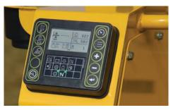
AT YOUR FINGERTIPS. An industry-unique on-machine control system offers the operator a variety of machine information, including pile angle and height. Display also shows machine maintenance reminders to help maintain service schedules.
