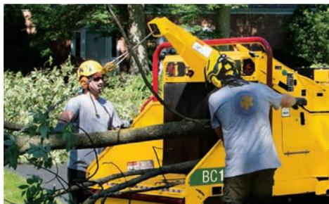
**EASILY LIFT HEAVY MATERIAL.** An optional winch allows operators to move large logs effortlessly. The 150' (45.7 m) winch line can handle logs up to 2000 lb (907.2 kg) and can automatically lift the logs onto the feed table.
