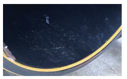
**POLYMER LINER.** The polymer liner inside the debris tank on the bottom half makes for efficient dumping and cleanout.
