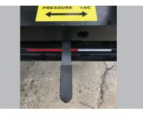
**REVERSE PRESSURE.** Reverse pressure to offload liquids and dislodge debris in hose.
