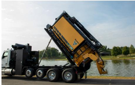
**WEIGHT.** Elongated spoil tank design with even weight distribution makes it the lightest vacuum truck in its size class. The spoil tank has a full-open cam-over rear door and lifts to a 50-degree angle for quick offloading.
