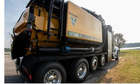
**SIDE STOW BOOM.** Side stow boom allows for quick jobsite setup by allowing the dig tube to always stay connected.
