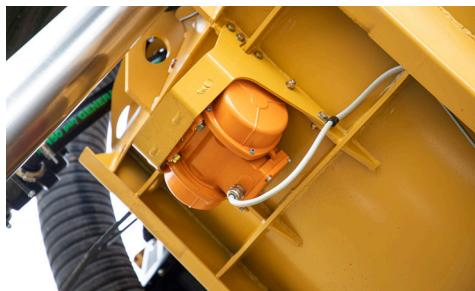
**SPOIL TANK VIBRATOR.** Optional vibrator allows for a more efficient way of dumping.
