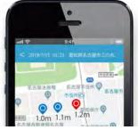
VERIFIER G3+ MAP MOBILE APP. Pair your smartphone with the locator to plot location information such as depth, current index, GPS data, operator name, device name and utility type.
