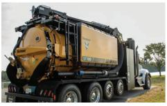
**SIDE STOW BOOM.** Side stow boom allows for quick jobsite setup by allowing the dig tube to always stay connected.
