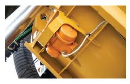
**SPOIL TANK VIBRATOR.** Optional vibrator allows for a more efficient way of dumping.
