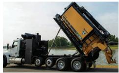
**WEIGHT.** Elongated spoil tank design with even weight distribution makes it the lightest vacuum truck in its size class. The spoil tank has a full-open cam-over rear door and lifts to a 50-degree angle for quick offloading.
