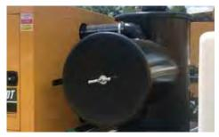
**CVS (CYCLONE 4-WAY VALVE SILENCER)** FILTRATION SYSTEM. .5-micron filtration. The CVS filter housing also contains the 4-way valve for reverse pressure and an oversized silencer for quiet operation. The silencer is located inside the 28-in (71-cm) diameter cyclone.
