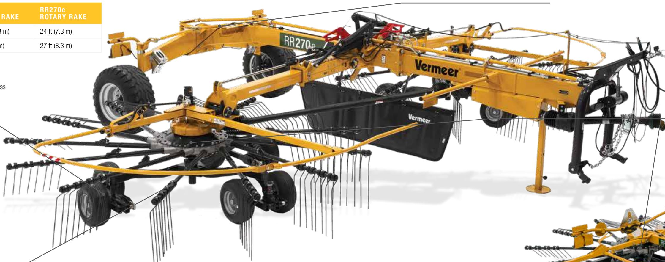
2 Optimal performance in the field comes from 13 tine arms on each rotor (12 on RR140s) — each designed to simplify maintenance and enhance operational efficiency. Cam and rake height have convenient toolless adjustments, allowing for precise control during operation. Additionally, each tine arm features a convenient lynchpin connection system for easy removal during transport or in case of damage.
