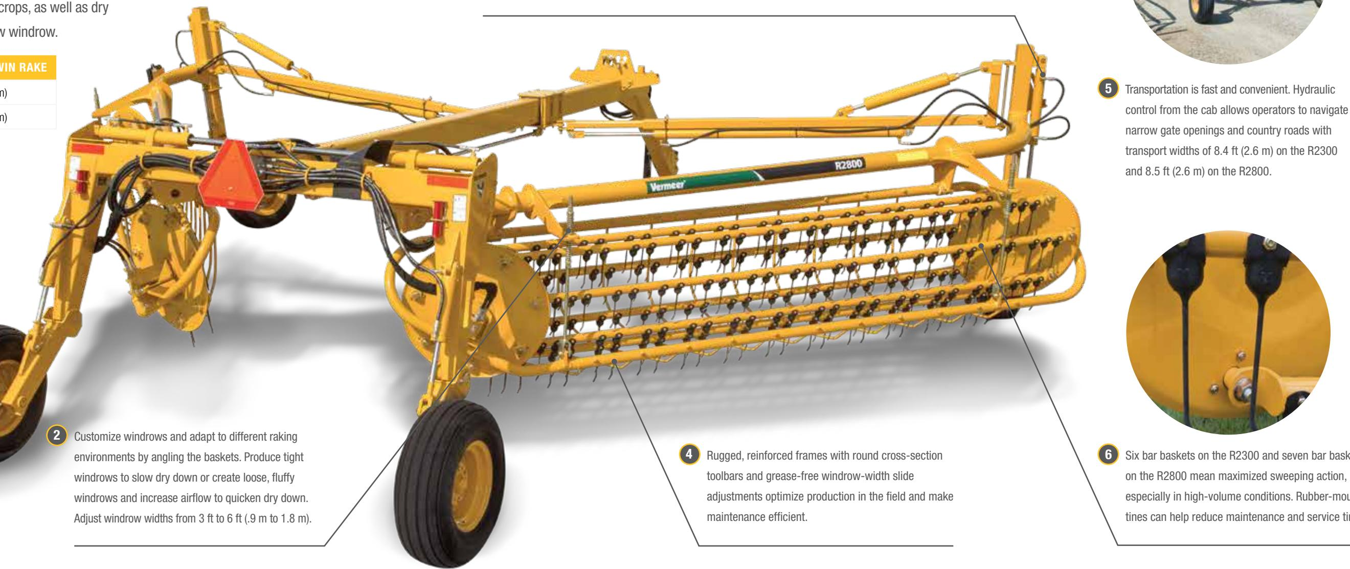
**3** Rake and windrow widths can be changed hydraulically to help maximize raking efficiency and customize windrow shape to your baler pickup.
