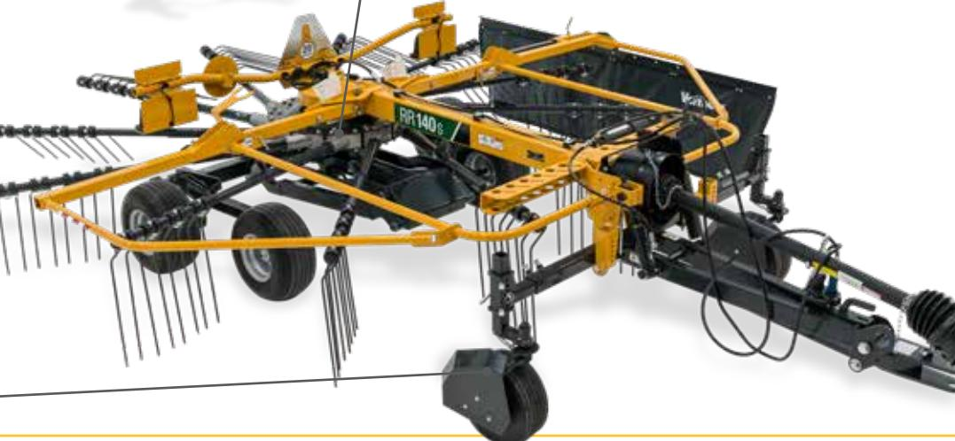
3 Enhance maneuverability and minimize field impact with a steerable axle ensuring the machine follows the tractor seamlessly during turns on the RR270c. The two-point hitch system connects to a robust linkage that allows the rear tires and axles to be adjusted independently of each other, optimizing raking performance and reducing footprint.
