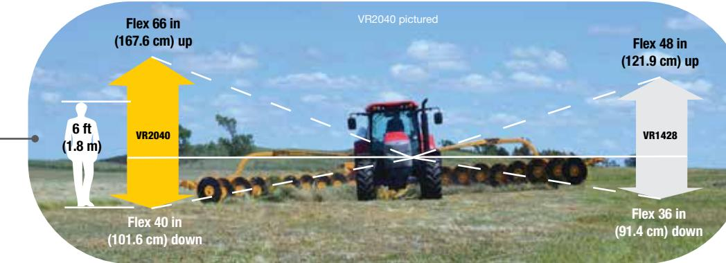
**4** One-piece rake arms and hydraulic suspension on each rake wheel provide flexibility with less maintenance than similar-sized rakes. Other rakes require a pivot joint and an additional caster wheel in the middle of the rake arm.
