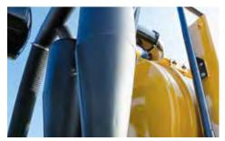
3-STAGE CYCLONIC FILTRATION. Designed specifically for 3,500 free air cfm (5,947 m<sup>3</sup>/hr) blower systems, it allows for wet and dry vacuum excavation while helping to prolong filter life and minimize maintenance costs.
