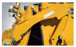
CAM-OVER REAR DOOR. The highly reliable cam-over design provides a 360-degree positive seal, with no additional clamping and no in-tank moving parts.
