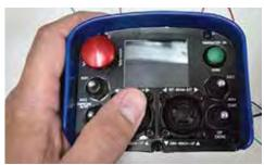
**FULL-FUNCTION, WIRELESS CAN BUS CONTROLS.** The radio remote monitors and controls all machine functions and vital information. Remote straps to the operator and features a machine stop.
