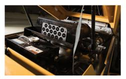
POWER FOR EVERY JOB. The RTX1250i2 is powered by a 127 hp (95 kW) Deutz TCD3.6L diesel engine which offers efficient power for working in difficult ground conditions.
