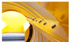
QUICK CHANGE SCREENS. Quick change screens can help improve job site efficiency, a particularly important feature when processing a range of materials that requires frequent screen changes.
