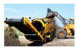
**CONVENIENT LOADING.** Large, low feed hoppers are easy to load without the need for loading ramps.
